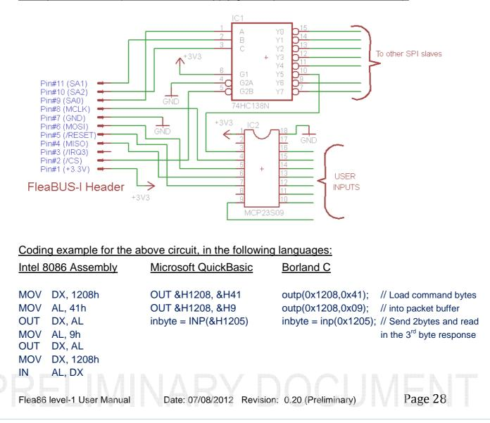
Example Schematic (Note: 74HC138 supply/ground pin connections not shown):
